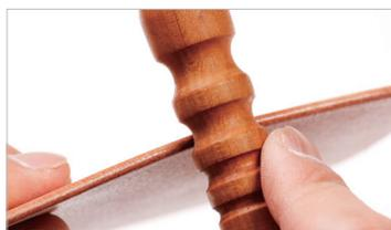
Apply to the flesh side or edge of leather, and work in with a burnishing tool until the desired finish is achieved. You can use "Slicker & Folder", "Glass plate", "Canvas", "Wooden slicker", "Wooden block" and so on as burnishing tools.
